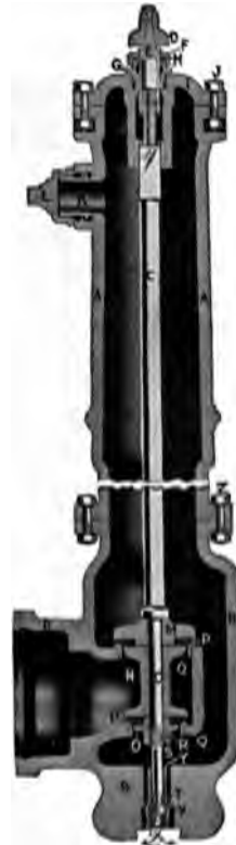
FIG. 142. — Ludlow Hydrant with Balanced Valve.
